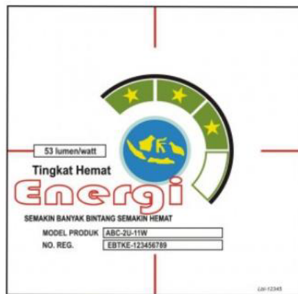
Figure 3: Indonesia energy efficiency label provides information on energy efficiency standards, model product number and registration number
