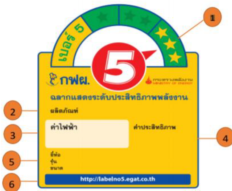
Figure 11: Thailand energy efficiency No.5 label (1: Energy efficiency level, the highest efficiency is 3 stars, 2: Indicates the type of product that has been certified, 3: Electricity bill per year to compare and estimate electricity usage, 4: Performance value for comparison with other products of similar size, 5: Product information, including brand, name, model, size, to be able to check the preliminary, 6: website of the Electricity Saving Label Project No. 5)
